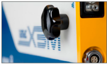
Locking screws when mounting on the antenna
